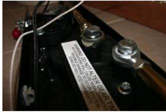
16. By operating the door leaves manually both leaves should achieve the fully open position (90°) at the same time. The aft door leaf must lead the forward door leaf during the closing operation. If this condition is not true, re-check each rigging step.
