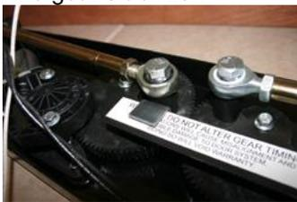
7. Connect the forward door push-pull rod (4) using the ½-20x1-3/4” bolt (19). The washer (20) must be placed between the rod end (3) and the actuator arm (2) or damage to the push-pull rod assembly (4) will result.
