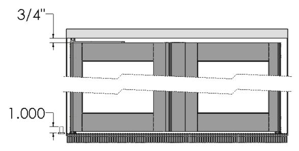
Example: The lower pivot shown here has a pin length of 1". The gap between the top of the door panel and the finished portal is 3/4" (Notice: this dimension is from the top of the aluminum frame of the door and not from any attachments on the door such as the torque arm). With the doors installed, there is no way for the door to be removed without removing the lower pivot.  $1" - \frac{3}{4}" = \frac{1}{8}$ " This installation conforms to the guidelines outlined in #11.
